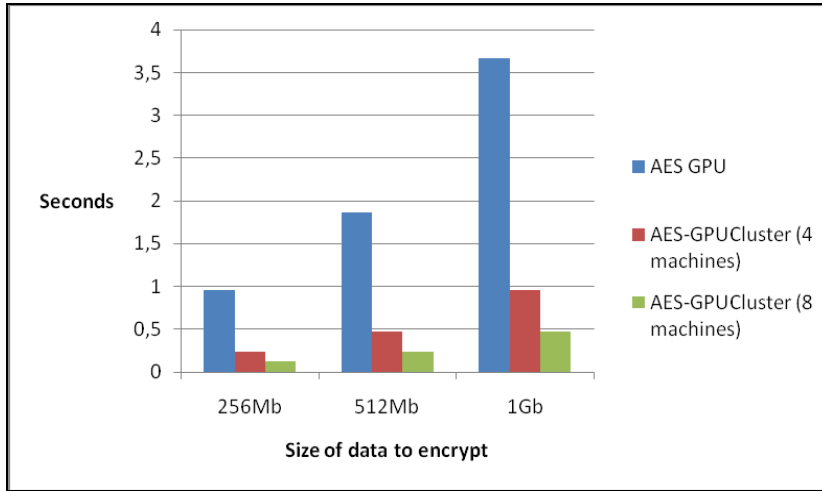
Fig. 3. AES-GPU time vs. AES-GPUCluster time (4 and 8 machines) excluding communications.
