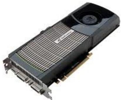
NVIDIA GeForce GTX480 (Fermi, 480 cores), 1.5GB GDDR5, 384-bits, compiled with gcc 4.1.1 (-O3 optimization) and CUDA 4.2.
